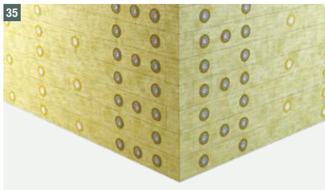
Outline for fixing MW lamellae (120×20 cm), 6 surface anchors, or 10 including the edge zone – Image 35
